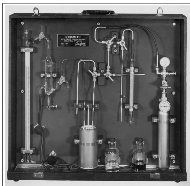
Figure 4. The Chromanette 9495 series portable GC of Podbielniak, based on the principle of Janák (21). On the right there is a lecture bottle of \text{CO}_2 used as the carrier gas. The chromatographic column is in the middle in a Dewar flask for thermostating. The nitrometer collecting the separated fractions is on the left.
