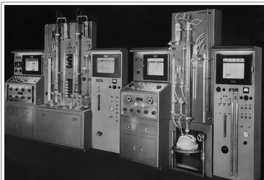
Figure 1. A publicity photo showing four Podbielniak instruments: (from left to right) the Thermocon 8700 series LTFD apparatus, a Chromacon 9400 series single-column GC, the Hyper-Cal 3700 series high-temperature fractional distillation apparatus, and a Chromacon 9400-V series multicolumn GC (21).
